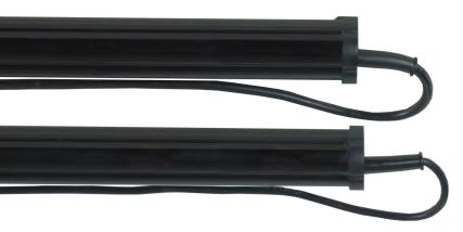
Using a series of thru beam photo eyes attached near the door track or guides, this light curtain is designed to provide a dense barrier of light that, when interrupted, signals the door to reverse. With the ability to span up to 32 feet wide and 6 feet high, it is suitable for use on the majority of commercial and industrial door applications.
